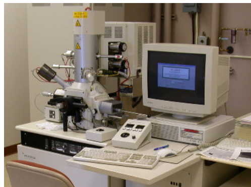
New Focused Ion Beam Milling system (Hitachi FB-2000A) in MTU's "Center for Nanomaterials Research".
